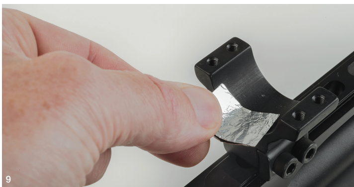
Fig.9: Put a strip of silver foil in the cradle of the rear mount to 'shim' the scope if the POI is initially a long way below the horizontal crosshair
