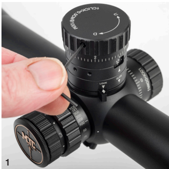
Fig.1 Loosen all screws on the turret cap
