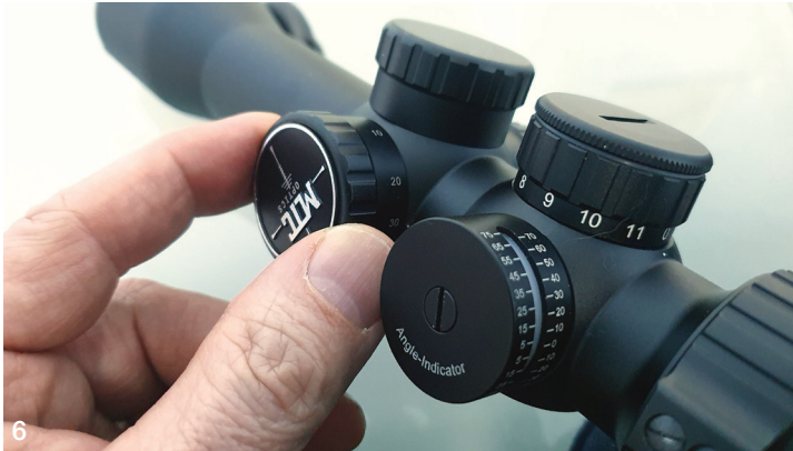
Figure 6: Turn the parallax side adjuster to ensure the target is at its sharpest. This will ensure any parallax error has been eliminated. The distance vernier can also be used as a rough range-finding guide.
