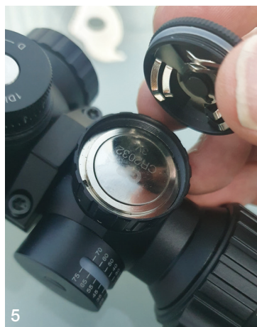
Figure 5: The CR2032 battery, accessed by unscrewing the rheostat cover
