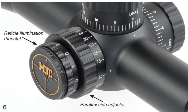
Figure 6: Turn the parallax side adjuster (inner ring) to ensure the target is at its sharpest. This will ensure any parallax error has been eliminated. The distance vernier can also be used as a rough range-finding guide. Note the outer ring, which is used to switch on and set the brightness level of the illuminated crosshair
