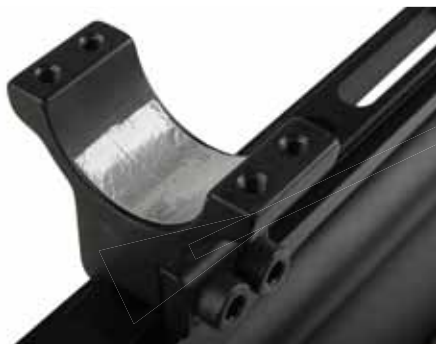
Figure 6: Shimming the rear mount
