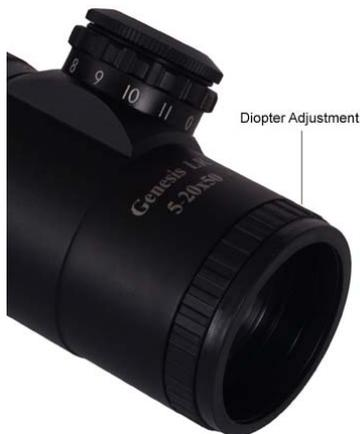
This obtains the sharpest Reticule image, and MUST be carried out first. This adjustment only needs to be carried out once and is unique to each user's eye. Rotate fast focus ring to get the sharpest possible reticule. Hint: Don't look at the Reticule for more than a few seconds at a time as your eye will compensate for less than perfect sharpness. Look away and look back again. Repeat until as sharp as possible.
