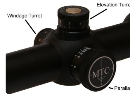
Access to the adjustment is gained by removing the covering caps. The adjusters are finger adjustable. The bullet strike is marked with up/ down (top turret) and left/right (side turret), i.e. if you want the bullet to go higher, turn anti-clockwise in the direction marked "up"
